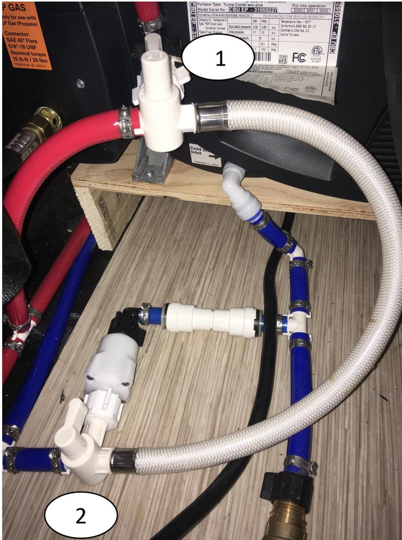
Valves are located under access panel beneath drivers-side bed. Valves shown in heater mode. To bypass heater turn both valves one quarter turn.
