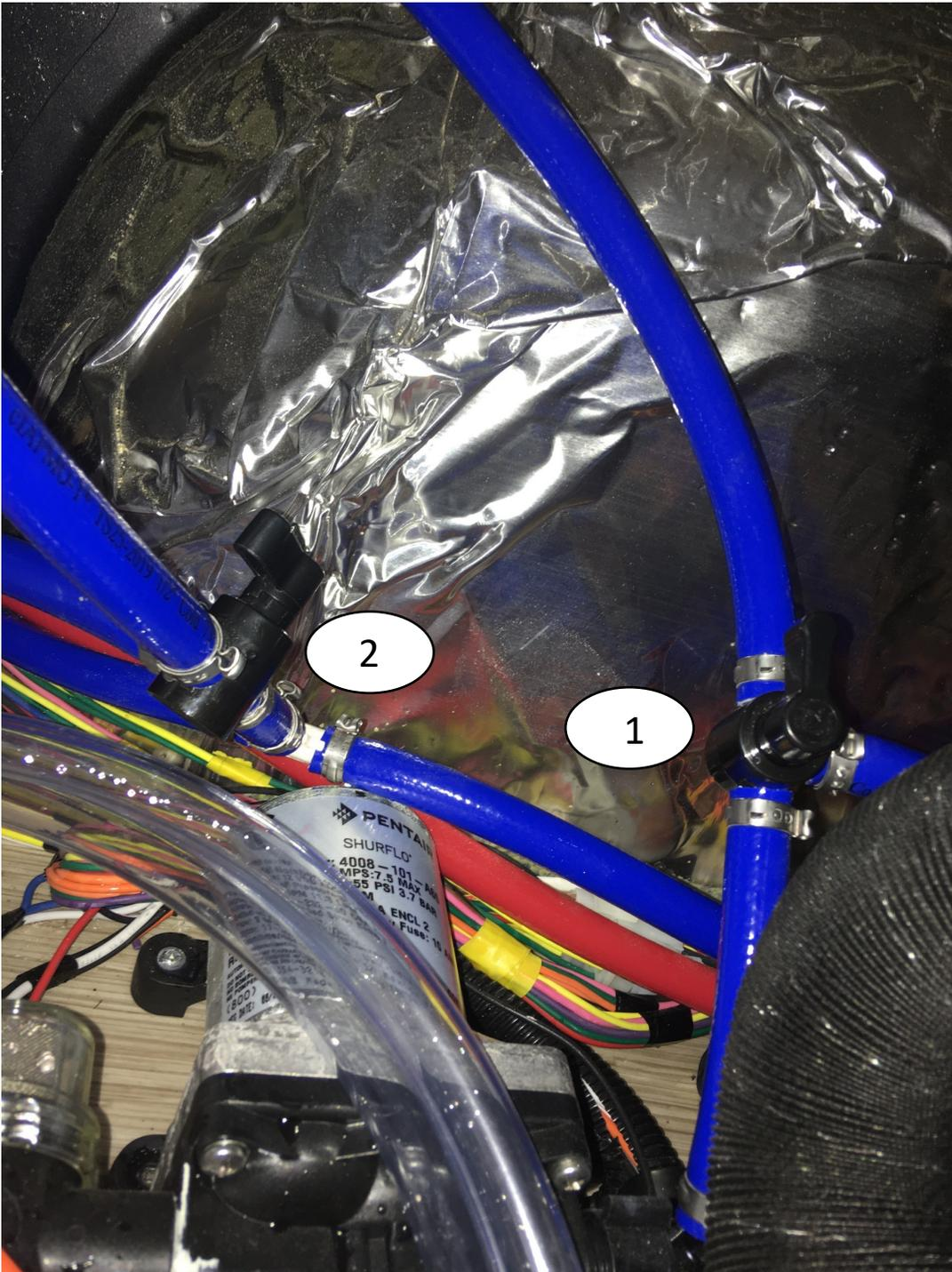
Valves are located behind side panel under the bed. Valve 1 – selects potable water source. Shown in on-board tank position. Turn valve clockwise one quarter turn to select city water.
