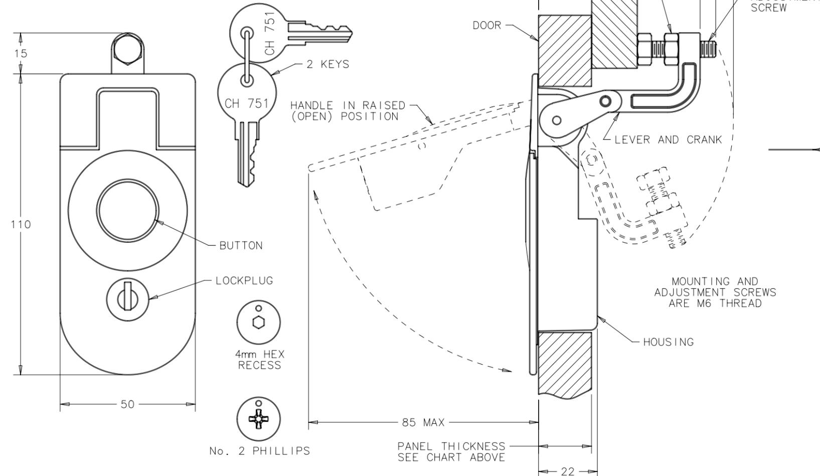
C5 SEALED LEVER LATCH WITH KEY OR TOOL ACCESS LOCKS
